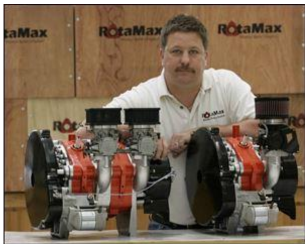
Eric Barger heads Thermo Fan, which makes a twin-rotor RotaMax engine, left, and a single-rotor model.
