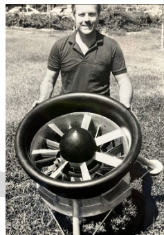
Airforce Drone with 530cc Rotapower® engine weighs 110 lbs. with payload of 95 lbs. and 125 miles range
