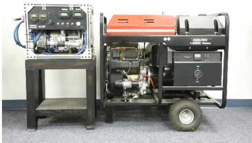
150cc Rotapower® engine genset weighs 65 lbs. and produces 15 Kw compared to Gillette genset weighs 395 lbs. and produces 13.5 Kw
